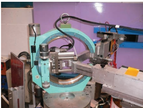
Figure 2.10. Tensile device adapted on the Euler cradle for in situ neutron diffraction measurements.
