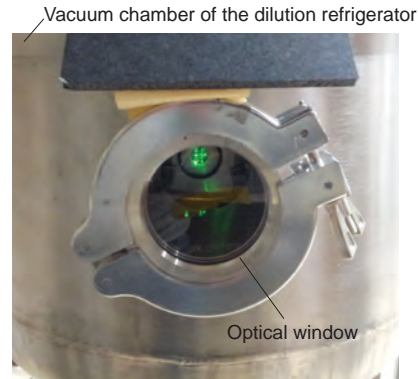
Figure 5.2: The optical access. The laser beam enters in the vacuum chamber of the dilution refrigerator via an optical window, and is aligned to hit the diamond region above the inductance of the resonator.
