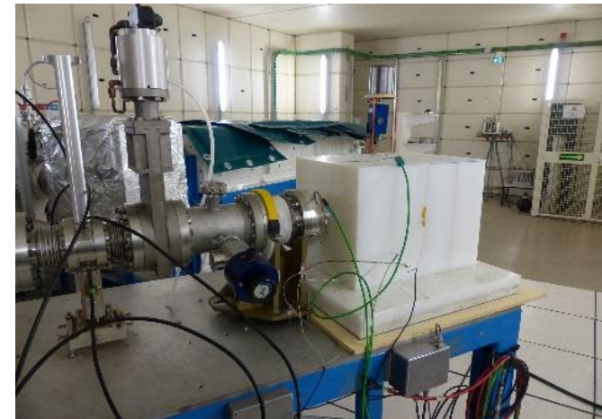
The polyethylene block around the Be target
