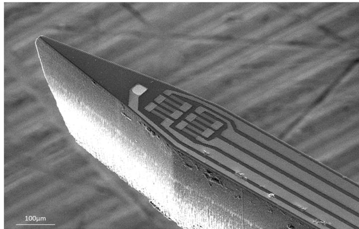
Figure 1: Sharp magnetorod with two GMR elements and an electrode
