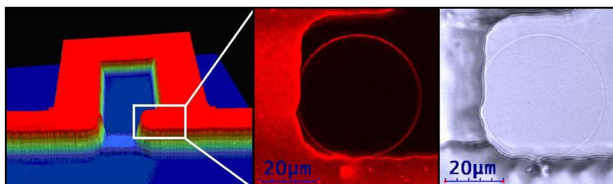
Left: optical interferometry 3D picture of the microfluidic trap. Middle: laser scanning confocal microscopy of a trapped vesicle. Right: the same vesicle observed with oblique illumination.
