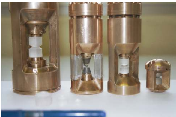
High pressure cells developed by Igor Goncharenko for neutron/X-ray scattering.
