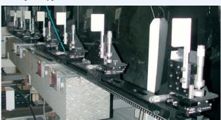
Figure 1. Picture of the prototype multi beam collimator with 7 masks
