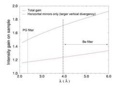
Figure 3. Calculated gain with supermirrors as a function of wavelength in two different configurations (see text).
