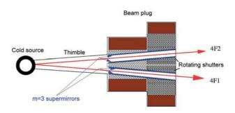
Figure 2. Schematic view of the cold source, thimble and beam plug assembly.
