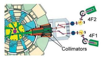
Figure 1. Setup of 4F1 4F2 cold triple axis spectrometers around the Orphée reactor.
