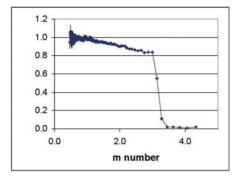
Figure 4. Neutron reflectivity measurement of one of the supermirrors inserted in the beam plug.
