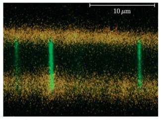
**Figure 3** (from Ref.2). PVDF membrane obtained by heavy ion irradiation and ion-track etching. Radicals that persist in nanopores after etching allows us a selective radiografting of poly(acrylic acid). Then a selective pore labelling with fluorophore is possible. The image the *xz*-plan cross-section of the membrane obtained by confocal laser scanning microscopy.
