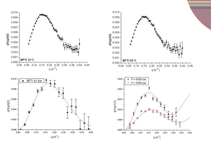
Figure 2 : Kratky plot of SANS spectrum for BPTI at ambient and high temperature (top) and at atmospheric pressure and high pressure (bottom).
