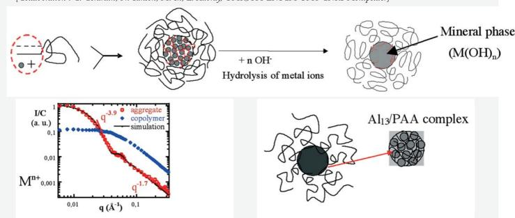
Comparison of SANS curves: Polymer alone (blue) and aggregate (red) of Al<sub>13</sub> + PAA 1900 -b- PHEA 8200, at the same polymer concentration.
