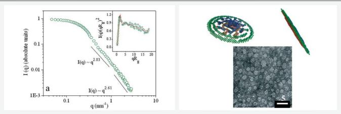
Form factor (SANS) of F1 at 25°C in D2O 50 mM NaCl, ab initio model and cryoTEM picture
