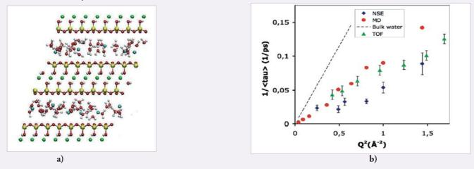
Figure 1. a) Atomic structure of a hydrated clay used in MD. Mobile species: water molecules (white and red), Na<sup>+</sup> / Cs<sup>+</sup> ions (blue). b) Inverse relaxation times versus the wave-vector for two-layer hydrate of Na-montmorillonite.
