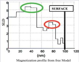
Figure 1: polarized neutron reflectivity of an SiC:Fe sample measured at 10K (fits in solid lines)
