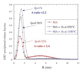
Figure 2 : Y<sub>2</sub>O<sub>3</sub> size distribution evolution under thermal treatment.
