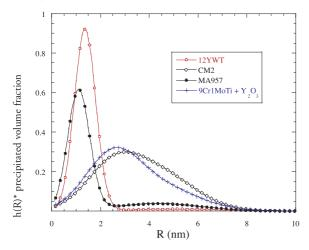
**Figure 1 :** Y<sub>2</sub>O<sub>3</sub> clusters size distribution in consolidated ODS alloys.
