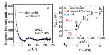
**Figure 3.** a. Magnetic intensity for x=0.2 sample at 1.4 K and 3.7 GPa. Lines are fits using SRO model and Lorentzian fit respectively. b. Phase diagram for  $(Tb_{1.x}La_x)_2Mo_2O_7$  in the threshold region: ambient pressure (open symbols) and under pressure (full symbols).
