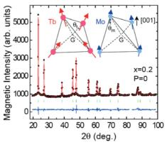
**Figure 2.** Magnetic intensity for x=0.2 at 1.5 K versus the scattering angle 2q,  $\lambda$ =2.426 Å. A 70 K spectrum was subtracted. Solid lines show the best refinement and the difference spectrum (bottom). In inset: magnetic structure of the Tb- and Mo- tetrahedra.
