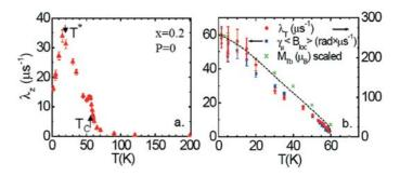
**Figure 4.**  $\mu$ SR ambient pressure results for x=0.2. Temperature dependence of: a.  $\lambda_{\gamma}$ . b. <B<sub>lor</sub>>,  $\lambda$ T and M<sub>Th</sub> (scaled).
