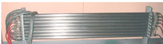
Figure 5. Test assembly of 8 linear-sensitive detectors.
