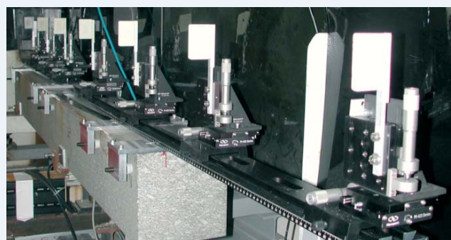
Figure 1. Picture of the prototype multi beam collimator with 7 masks
