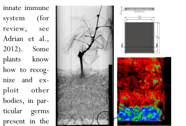
Figure 4: Neutron images of a grapevine herbaceous cutting cultivated by the AgroEcology team (Dijon) in an aluminium flat container (LLB design, Helary A.). The left « black and white » image has been performed with an image plate detector (neutronography station G4.5) and the right color one comes from the IMAGINE station (40 s of exposure), with
