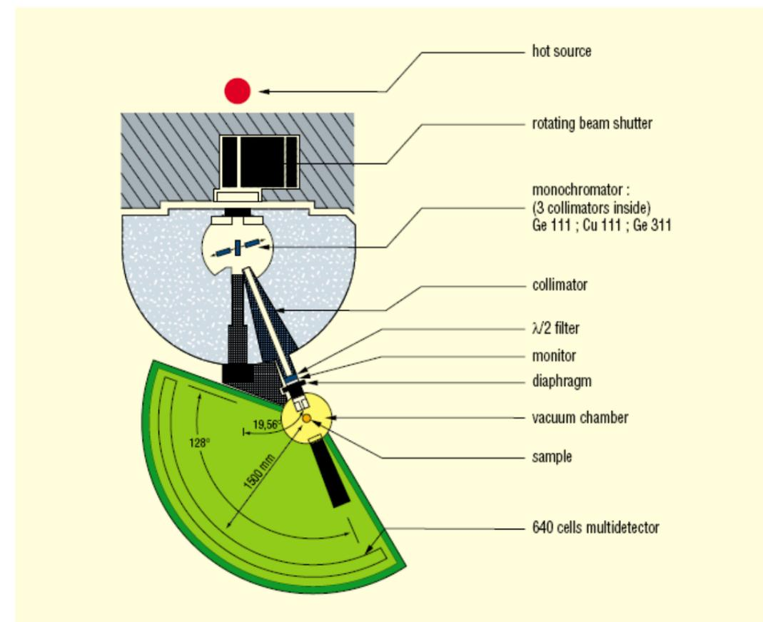
**General layout of the diffractometer 7 C2.**
