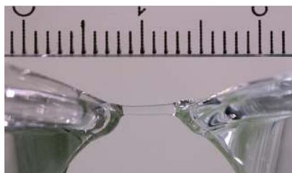
Water bridge (5mm length, 1mm diameter) between two glasses filled with heavy water, under a voltage of 15 kV.
