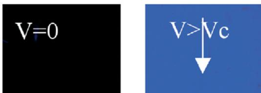
Above a critical shear rate, the isotropic liquid of liquid crystal polymers (left photo) transforms in a strongly birefringent oriented phase (right photo). Photos are obtained between crossed polarisers in the (velocity, neutral axis) plane.
