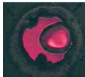
Figure 1. Single crystal of solid D_2 surrounded by He pressure transmitting medium.
