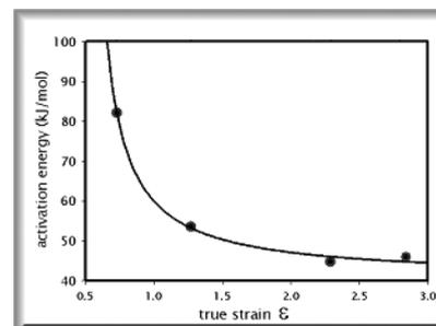
Figure 4. Evolution of activation energy  $E_a$  as function of the true strain.
