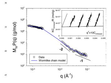
**Fig. 1** Combined static light scattering and SANS spectra for a 0.1g/l chitosan solution. To superimpose both techniques we plot M<sub>w</sub>P(q) as a function of q. The continuous line represents the fit of the data with a <sup>50</sup> wormlike chain model (see ESI). The Zimm plot of chitosan is presented in the inset.
