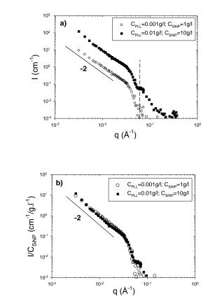
Fig. 6 (a) SANS spectra obtained for Poly-L-lysine (PLL)/SiNP solutions in domain #3 (excess of NPs) in the presence of 0.2 M KBr. (b) same as  $_{95}$  (a) but representation of the variation with q of the ratio I/C<sub>SiNP</sub>.
