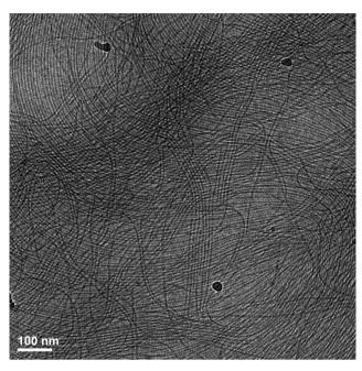
Fig. 5 CryoTEM for monomer B1\* solution (0.25% in water).
