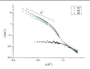
**Fig. 7** SANS intensity (*I*) versus scattering vector (*q*) for monomer **B1**<sup>\*</sup> and oligomers **B2** and **B3** solutions in CD<sub>3</sub>OD at 10 g L<sup>-1</sup> and 25 °C.
