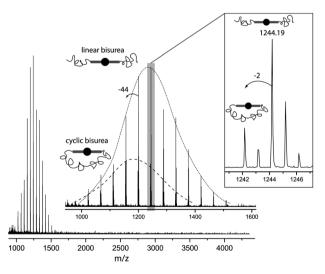
Fig. 3 MALDI-TOF spectrum for oligomer B3.
