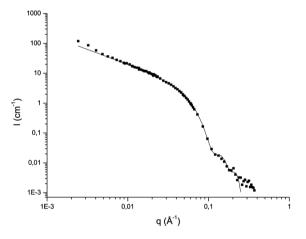
**Fig. 6** SANS intensity (*I*) versus scattering vector (*q*) for monomer **B1**\* solution in  $D_2O$  at 10 g L<sup>-1</sup> and 25 °C. The plain curve is a fit according to a model for two populations of long rigid filaments with a circular cross-section (respective cross-section diameters: 5.6 and 7.5 nm).
