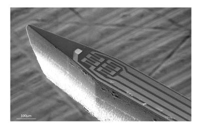
Figure 1: Sharp magnetrode with two GMR elements and an electrode
