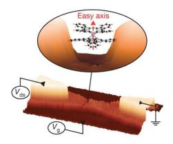
Three-dimensional extrapolation of a scanning-electron-microscope image showing the most favourable structure of the single-molecule-based transistor. A schematic zoom into the nano gap shows the molecular structure of the TbPc2 SMM and its easy axis. The charge state of the ligand read-out dot can be controlled by the gate voltage, Vg, and the voltage difference between the electrodes is controlled through the drain-source voltage, Vds
