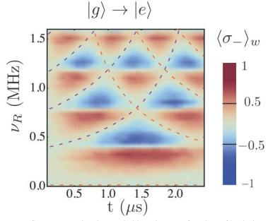
Resonance fluorescence signal, encoded in color, as a function of both time and Rabi frequency, for qubit prepared in  $|g\rangle$  and post-selected in  $|e\rangle$ .
