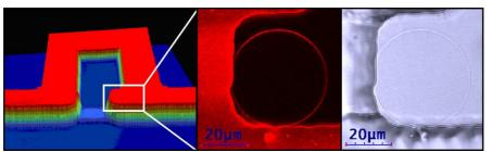
Left: optical interferometry 3D picture of the microfluidic trap. Middle: laser scanning confocal microscopy of a trapped vesicle. Right: the same vesicle observed with oblique illumination.
