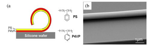
**Fig.1** (a) Structure of a polymer bilayer which undergoes self-rolling in a water solution of an alcohol or an acid. (b) Scanning electron microscopy of a micron-wide tube.
