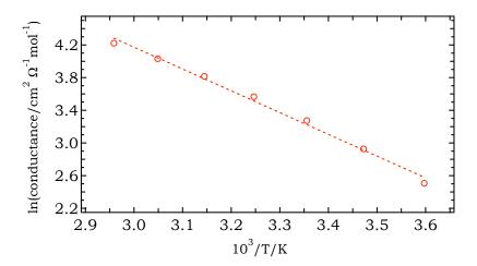
**Figure** of 23kJ4.8: Estimation activation energy  $\mathbf{mol}^{-1}$ of  $TBA^+$ mobility **TBABr** soluaqueous tions from conductivity (data taken measurement from [Eagland 1972] [Buchner 2002] [Surdo 1979]).
