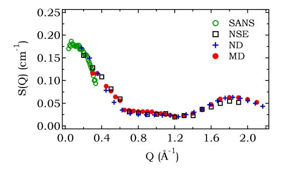
Figure 7.6: Scattered coherent intensity (cm<sup>-1</sup>) as a function Q of the aqueous TBABr solution with  $x_m$ =1:56 by different techniques. The agreement of our MD simulation result with experiments covers a large Q range.
