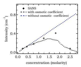
Figure 7.10: Extrapolated SANS intensity at Q=0 as a function of concentration for aqueous TBABr solution with  $x_m=1:56$ . The theoretical prediction with and without the effect of osmotic coefficient is shown.
