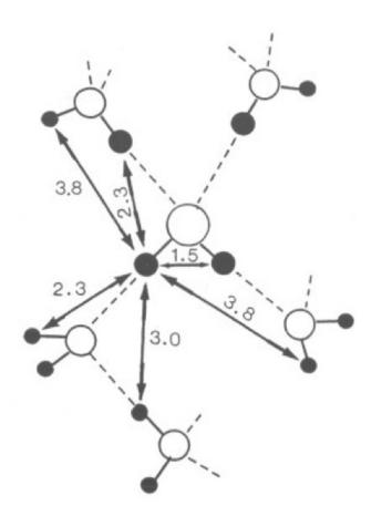
Figure 4.10: Structural geometry of hydrogen bonding in water molecules and its nearest neighbors (distance in Å). white - oxygen atom, black - hydrogen atom [Turner 1990].
