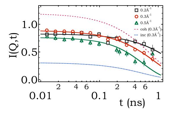
Figure 8.7: Intermediate scattering functions  $I^{NSE}(Q,t)$ , measured by NSE, for 3 different wave-vectors in the low-Q region (Reseda spectrometer). The signal for Q=0.3 Å<sup>-1</sup> is decoupled into the coherent and incoherent contribution.
