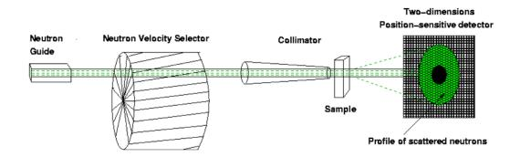
Figure 5.4: Schematic diagram of Small Angle Neutron Scattering spectrometer.
