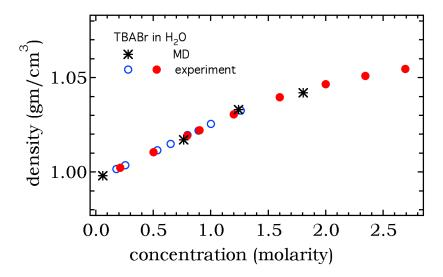
Figure **6.2**: Comparison density TBABrof of aqueous solution extracted MDsimulation from and experiment [Buchner 2002] [Eagland 1972].
