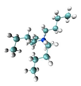
Figure 4.1:  $TBA^+$  ( $C_4H_9$ ) $_4N^+$  cation (blue - nitrogen, green - carbon and white - hydrogen atom). The hydrophobicity can be modified by changing the length of the hydrocarbon chains. This is one fundamental difference with simple inorganic ions where electrostatic interaction is the sole deciding factor.
