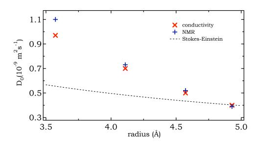
Figure 4.7: Comparison of TAA cation translational diffusion coefficient at infinite dilution extracted from experiment (NMR and conductivity) and Stokes-Einstein relation. As the cation size increases the agreement between Stokes-Einstein and experiment becomes better.
