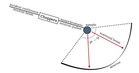
Figure 5.6: Time of Flight spectrometer.
