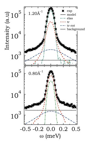
Figure 8.4: Incoherent scattering functions,  $S_{inc}(Q,\omega)$ , versus energy transfer for Q=1.20 Å<sup>-1</sup> (top) and Q=0.80 Å<sup>-1</sup> (bottom) measured by TOF. Different components of the model function are shown: background (dashed black), elastic (green), translational (red), trans-rotational (blue) and total (full black).
