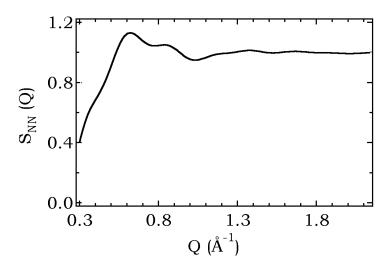
Figure 7.9: Calculated partial structure factor of TBA<sup>+</sup> central nitrogen  $S_{NN}(Q)$  as a function Q, shows constant value and a small peak around Q=0.65 Å and then steadily decreases towards lower Q indicating the presence of some interaction. Nitrogen (N) is the CoM of TBA<sup>+</sup>.
