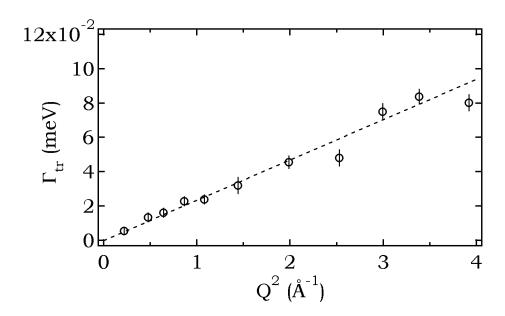
Figure 8.19:  $\Gamma_{tr}$  from TOF measurement for aqueous TBABr solution with  $x_m$ =1:112 is plotted as a function  $Q^2$ . The translational diffusion coefficient  $D_{tr}$  is calculated from a linear fit passing through origin (continuous diffusion).
