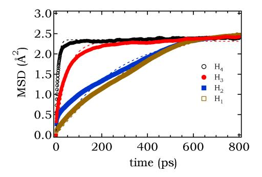
Figure 8.18: MSD of different hydrogen atoms (with modified coordinates relative to its central carbon) of TBA<sup>+</sup> as a function of time. The suffix of different hydrogens are named after each carbon atom in alkyl-chain.
