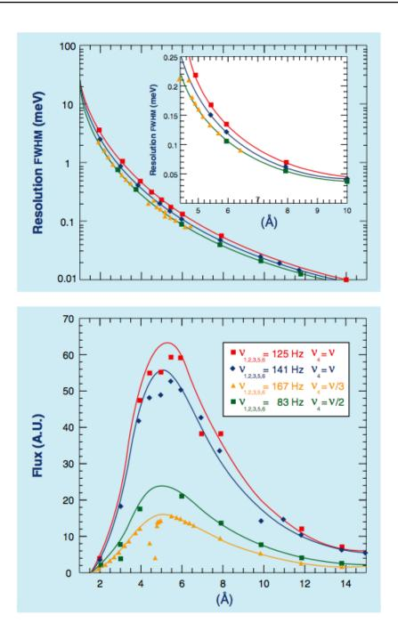
Figure 5.7: Plot of Resolution and Flux as a function of incident neutron wavelength of Mibemol TOF spectrometer. The resolution is a slowly varying function while the flux depends strongly on the wavelength. Here is an example for four frequencies of the 6 choppers. Except 4 (this is anti-over lap chopper), the frequencies of all other choppers are indicated in the figure (www.llb-cea.fr).
