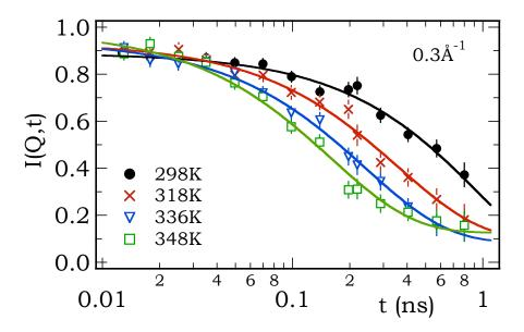
Figure 8.32: The temperature dependence of the intermediate scattering function measured by NSE,  $I^{NSE}(Q,t)$ , for Q=0.3Å<sup>-1</sup> on aqueous solution of TBABr with  $x_m$ =1:56 (Reseda spectrometer).
