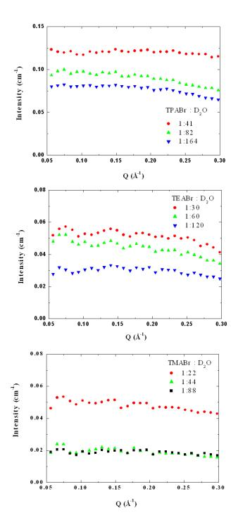
Figure 7.4: SANS coherent intensity (in  $cm^{-1}$ ) versus the wavevector Q, for a series of different aqueous TAABr solutions. From top to bottom, TPABr, TEABr and TMABr are in  $D_2O$ . No sign of aggregation is observed.
