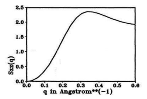
Figure 4.2: Charge-Charge structure factor  $[S_{ZZ}(Q)]$  as a function of Q for 0.25M  $Et_3PhN^+Ph_4B^-$  in DMF [Kunz 1992a].
