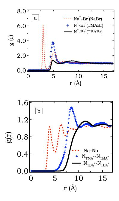
Figure 7.7: Ion-ion radial distribution function of the aqueous TBABr, TMABr and NaBr solution with  $x_m=1:56$ . (a) how bro-mide anion is associated to different cations and penetration in case of TBA<sup>+</sup> (b) Some interaction is present around 11 Å for TBA<sup>+</sup> cation which is largely nullified by presence of oppositely charged anions.
