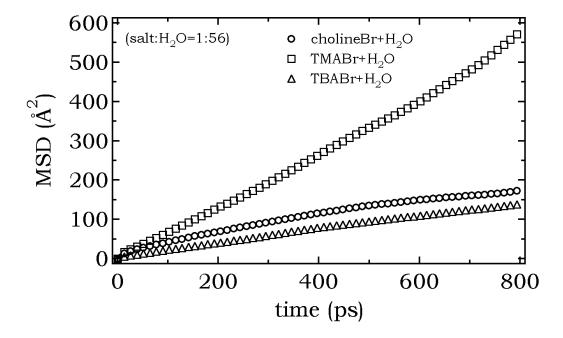
Figure 8.24: The MSD of average hydrogen atoms of TMA<sup>+</sup>, Choline<sup>+</sup> and TBA<sup>+</sup> cations are plotted as a function of time for aqueous solution with  $x_m$ =1:56.
