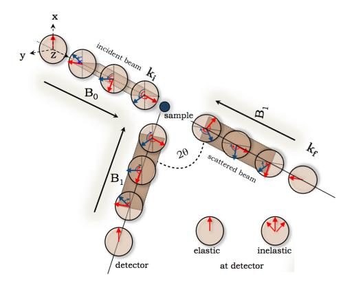
Figure 5.11: Classical Neutron Spin Echo technique.
