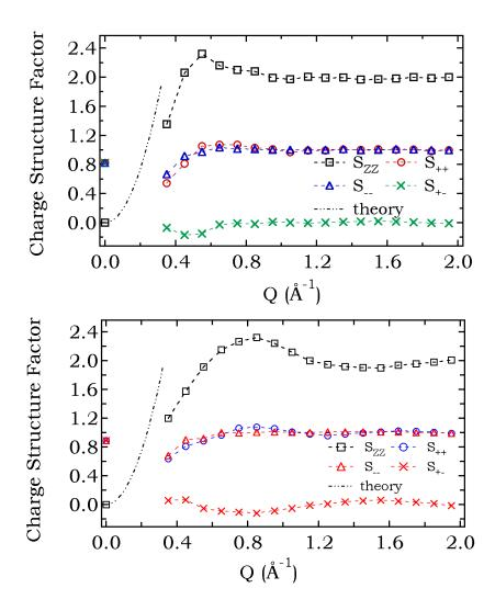
Figure 7.11: Partial  $(S_{ij}(Q))$  and total  $(S_{ZZ}(Q))$  charge-charge structure factor for TBABr (upper) and TMABr (lower) as a function of Q. At Q=0,  $S_{ZZ}(0)$ =0 and  $S_{ij}(0)$ = S(0). At finite Q value the non-zero value of  $S_{ZZ}(Q)$  suggests that an ion charge is not completely screened by other ions. The estimated  $S_{ZZ}(Q)$  at  $Q < \kappa$  is also plotted in the same graph (denoted by theory).
