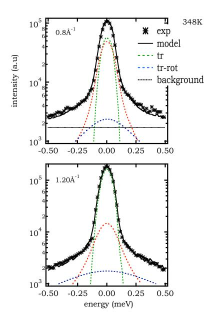
Figure 8.28: Incoherent scattering functions,  $S_{inc}(Q,\omega)$ , versus energy transfer for Q=1.20 Å<sup>-1</sup> (top) and Q=0.80 Å<sup>-1</sup> (bottom) measured by TOF at 348K on aqueous solution of TBABr with  $x_m$ =1:56. Different components of the model function are shown: background (dashed black), elastic (green), translational (red), trans-rotational (blue) and total (full black).
