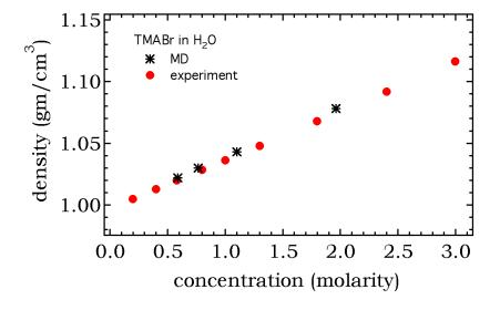
Figure 6.3: Comparison of density of aqueous TMABr solution extracted from MD simulation and experiment [Buchner 2002].
