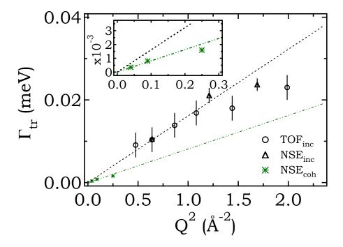
Figure 8.8: Translational broadening,  $\Gamma_{tr}$ , extracted from the incoherent and coherent signal is plotted as a function of  $Q^2$ . The broadening  $\Gamma_{tr}$  corresponds to the translational relaxation time,  $\Gamma_{tr} = \frac{\hbar}{\tau_{tr}}$ . The straight lines correspond to linear fits of the incoherent and coherent broadening from which the corresponding diffusion coefficients were determined. Insert: A zoom of the low Q region.
