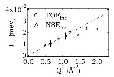
Figure 8.5: Translational broadening,  $\Gamma_{tr}$ , versus  $\mathbf{Q}^2$  extracted from the incoherent signal in the middle Q region by as measured by TOF and NSE.
