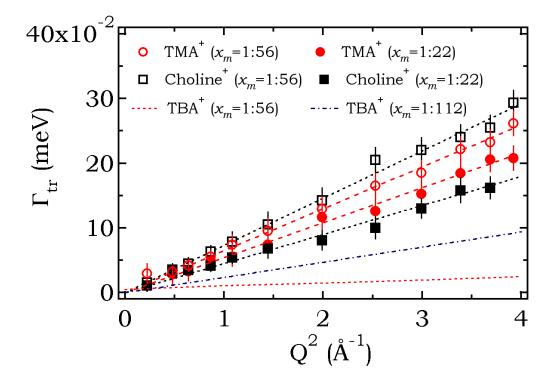
Figure 8.23:  $\Gamma_{tr}$  extracted from TOF measurement for different cations at different concentrations, are plotted as a function  $Q^2$ . The translational diffusion coefficient  $D_{tr}$  is calculated from a linear fit passing through origin (continuous diffusion).
