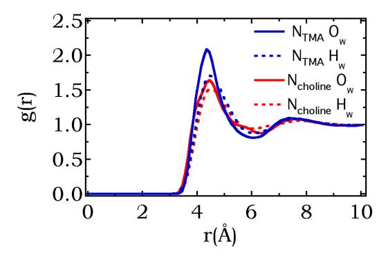
Figure 9.2: Cation-water Radial Distribution Function for aqueous TMABr and CholineBr solutions with  $x_m=1:56$ .
