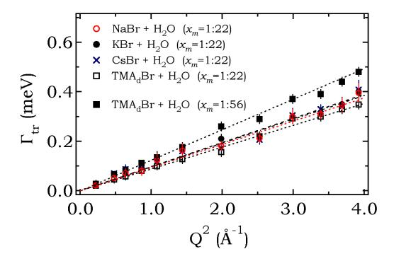
Figure 9.7:  $\Gamma_{tr}$  from TOF measurement is plotted as a function  $\mathbf{Q}^2$  to extract the  $\mathbf{D}_{tr}$  of average solvent water molecules from a linear fit passing through origin (continuous diffusion).
