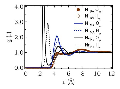
Figure 9.1: Cation-water Radial Distribution Function of aqueous TBABr, TMABr and NaBr solutions with  $x_m=1:56$ , to show how the hydration water is structured differently as we move from simple (such as NaBr) to hydrophobic salts (TMABr, TBABr)
