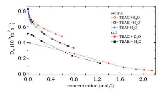
Figure 4.9: Self and mutual diffusion coefficient of aqueous TAA halide solution, estimated by different experimental techniques. The mutual diffusion coefficients are measured by optical diffusiometer. The self-dynamics of TBA cation is measured by NMR (Br anion) [Hertz 1969] and Tracer (Cl anion) [Woolf 1982] and mutual-dynamics by optical diffusion technique [Kim 1973].
