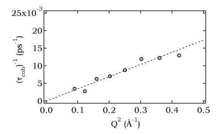
Figure 8.21: Inverse of translational relaxation time (extracted from simulated coherent I(Q,t) curves are plotted as a function of  $Q^2$  for aqueous TBABr solution with  $x_m=1:112$ . The  $D_{tr}$  from a linear fit passing through origin (continuous diffusion).
