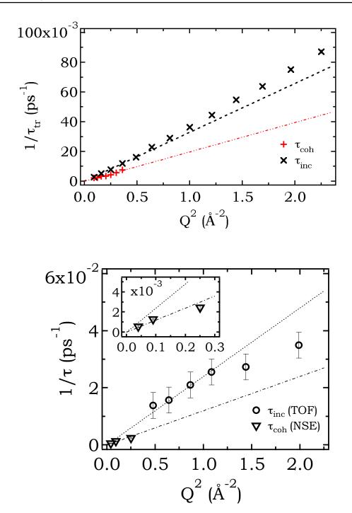
Figure 8.12: (top) MD simulation, (bottom) Neutron experiment. Inverse translational relaxation time plotted as a function of  $Q^2$ . The inverse relaxation times ( $\tau_{inc}$  and  $\tau_{coh}$ ) are extracted from exponential modelling of simulated/ experimental intermediate scattering functions corresponding to the incoherent signal and the total coherent signal.
