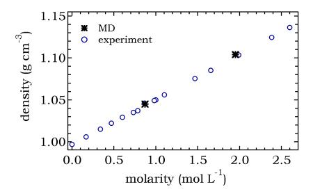
Figure 6.4: Comparison of density of aqueous CholineBr solution extracted from MD simulation and experiment.
