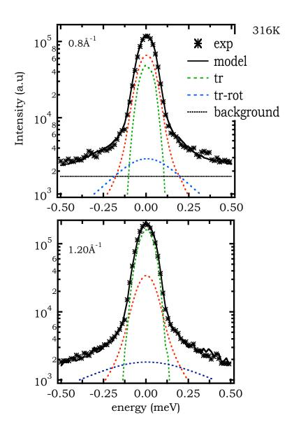
Figure 8.27: Incoherent scattering functions,  $S_{inc}(Q,\omega)$ , versus energy transfer for Q=1.20 Å<sup>-1</sup> (top) and Q=0.80 Å<sup>-1</sup> (bottom) measured by TOF at 316K on aqueous solution of TBABr with  $x_m$ =1:56. Different components of the model function are shown: background (dashed black), elastic (green), translational (red), trans-rotational (blue) and total (full black).
