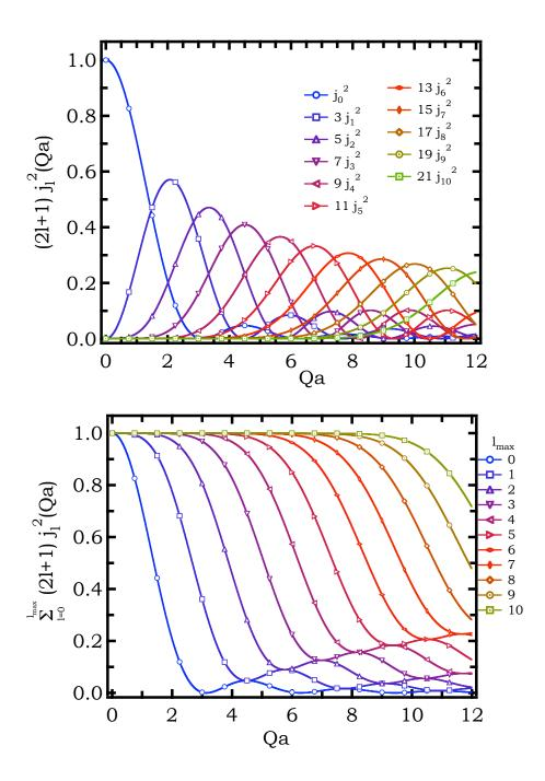
Figure 5.12: Change in the value of Bessel function is shown as a function of the product of Q (reciprocal wave vector) and a (radius). Top: each of the Bessel function (for l=0 to 10) is shown separately. Bottom: The sum of the Bessel functions are shown. The curves show that the first two orders  $j_0$  and  $j_1$  dominates over the higher terms at low value of Qa.
