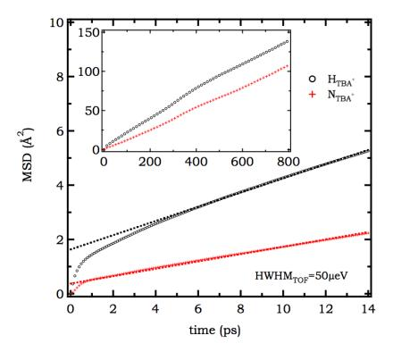
Figure 8.9: (a)  $D_{tr}$  extracted from MSD analysis of aqueous TBABr solutions with  $x_m$ =1:56. Difference between nitrogen (CoM) motion (red cross) and average hydrogen movement (black circle) in TOF time-window (14ps) is shown. insert: MSD of the same two quantities i.e. nitrogen (CoM) and hydrogen atoms but for a much longer time scale. Note the hydrogen MSD changes its slope after  $\sim$ 400ps.
