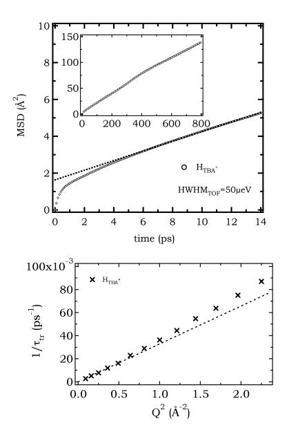
Figure 8.6: (top)  $D_{tr}$  extracted from MSD analysis of hydrogen atoms present in aqueous TBABr solutions with  $x_m$ =1:56. Note the hydrogen MSD changes its slope after  $\sim$ 400ps which indicates the global rotation time. (bottom) inverse translational relaxation time as a function of  $\mathbf{Q}^2$ .  $\mathbf{I}_{inc}(Q,t)$  of average hydrogen predicts an intermediate  $\mathbf{D}_{tr}$  as in MSD analysis.
