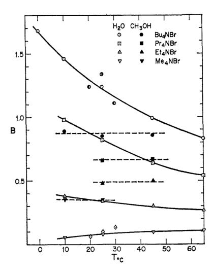
Figure 4.6: B coefficient of Jones-Dole equation for TAABr in water and methanol as a function of temperature. A clear difference can be observed for TBABr and for TPABr compared to TMABr with TEABr as neutral, after [Kay 1966b].
