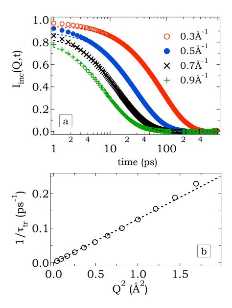
Figure 9.4: Dynamics of average solvent water molecule of TBABr solutions with  $x_m=1:56$ . (a)  $\mathbf{I}_{inc}(Q,t)$  of hydrogen atoms of water (b) Inverse translational time extracted from  $\mathbf{I}_{inc}(Q,t)$  versus  $\mathbf{Q}^2$ . The slope corresponds to the  $D_{tr}$  of solvent water.
