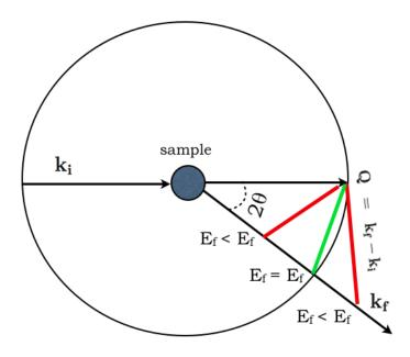
Figure 5.2: Elastic and inelastic scattering as incident wave vector scatters through an angle  $2\theta$ .
