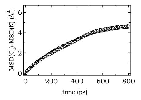
Figure 8.15: Estimation of global rotation time of TBA<sup>+</sup> by MSD analysis. The difference of MSD between carbon (attached directly to central nitrogen) and nitrogen (CoM) atoms are calculated which provides the global rotation time. The fitting equation is  $2b^2(1-e^{-\frac{t}{\tau_{rot}^{glob}}})$ , where  $\tau_{rot}^{glob}$  is the global rotational time and b is the nitrogencarbon bond length.
