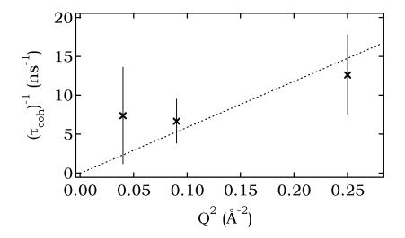
Figure 8.22: Inverse of translational relaxation time extracted from NSE coherent I(Q,t) curves is plotted as a function of  $Q^2$  for aqueous TMABr solution with  $x_m=1:22$ . The  $D_{tr}$  is extracted from a linear fit passing through origin (continuous diffusion).
