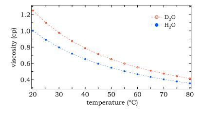
Figure 4.12: Viscosity of  $H_2O$  and  $D_2O$  as a function of temperature.
