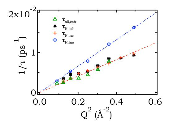
Figure 8.14: Inverse relaxation times, plotted versus  $Q^2$ , extracted from exponential modelling of simulated intermediate scattering functions corresponding to (a) the total coherent signal  $(\tau_{coh}^{all})$ , (b) correlations (self and distinct) between central N atoms of the cations  $(\tau_{coh}^N)$ , (c) self-correlations of the central N atoms of the cations  $(\tau_{inc}^N)$  and (d) self-correlations of the H atoms of the cations  $(\tau_{inc}^H)$ .
