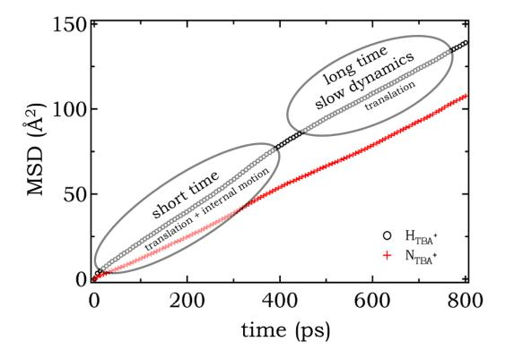
Figure 8.13: MSD of the TBA $^+$  hydrogen atoms as a function of time. Note that the hydrogen MSD changes its slope after  $\sim 400 \mathrm{ps}$ . The short time (less than  $\sim 400 \mathrm{ps}$ ) can be originated from global cation rotation, individual hydrogen rotation or alkyl chain internal motion.
