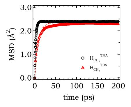
Figure 8.16: MSD of terminal methyl hydrogen atoms (with modified coordinates relative to its central carbon) as a function of time to extract methyl hydrogen rotation time ( $\tau_{rot}^{CH_3}$ ). Black circle (TMA<sup>+</sup> methyl hydrogen) and red square (TBA<sup>+</sup> methyl hydrogen).
