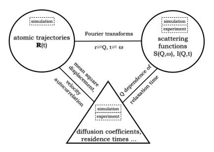
Figure 6.1: Calculation of diffusion coefficient from neutron experiment and MD simulation.
