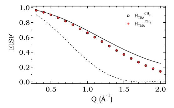
Figure 8.17: Elastic Incoherent Structure Factor (EISF) as a function of Q for methyl hydrogen of  $TMA^+$  and  $TBA^+$ . The solid line is  $A_0(Q)$  with r = 1.8 Å and dashed line is with r free.
