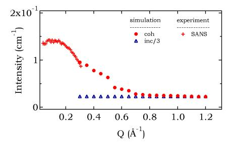
Figure 8.2: Decoupling of coherent and incoherent intensity as a function Q for aqueous TBABr solution with  $x_m=1:112$  (extracted by MD simulation). The coherent SANS signal is in agreement with the predicted simulated result.
