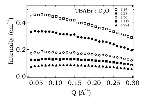
Figure 7.3: SANS coherent intensity (in cm<sup>-1</sup>) versus the wave-vector Q, for a series of aqueous TBABr solutions (with  $x_m$ =1:224 to 1:14). Error bars are smaller than symbol size. We do not see any aggregation as the concentration increases.
