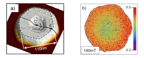
Figure 1: (a) Constant current STM image of the *Pb* island grown on Si(111) substrate that was selected for the study. (b) In non-zero magnetic field the tunneling spectra become spatially inhomogeneous over the island: the color-coded Zero-Bias Tunneling Conductance (ZBC) map of the island (here at H=180 mT) shows the radial distribution of ZBC values with higher ZBC observed close to the island border due to the pair-breaking effect of the circulating supercurrents.
