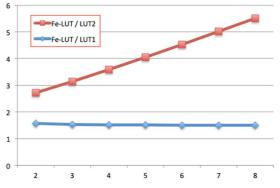
Fe-LUT improvement factor in overall transistor count compared to other FeFET-based LUTs, as a function of number of LUT inputs
