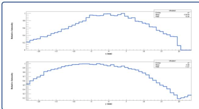
$$\sigma_x = 10.4 \text{ mm} - \sigma_y = 11.6 \text{ mm}$$
