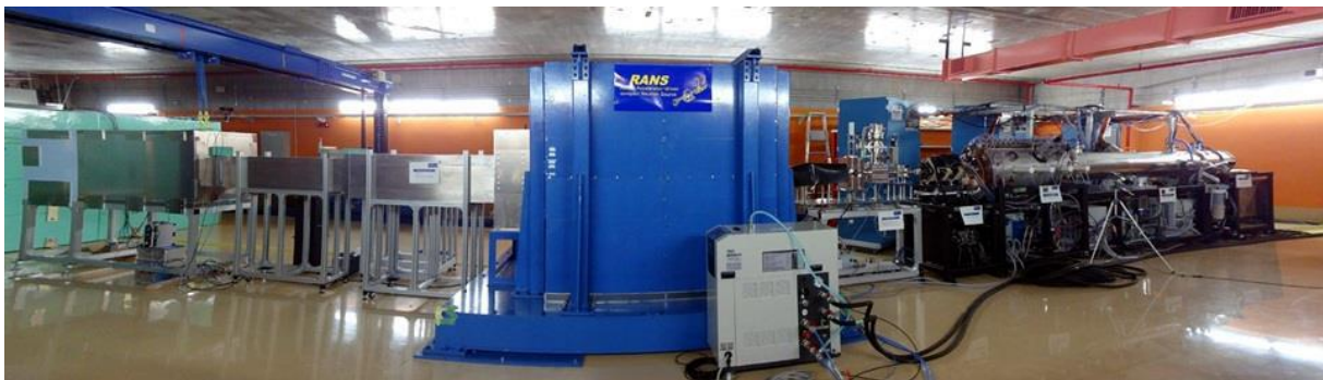
Figure 3: The RANS casemate. (left) scattering instrument (middle) TMR assembly, mostly shielding, (right) accelerator.
