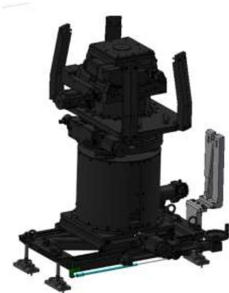
**Fig. 6** – View of the sample table. A custom pivot system (shown in gray) will allow rotating the detector vessel w.r.t. its center of rotation.
