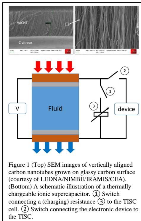
Figure 1 (Top) SEM images of vertically aligned carbon nanotubes grown on glassy carbon surface (courtesy of LEDNA/NIMBE/IRAMIS/CEA). (Bottom) A schematic illustration of a thermally chargeable ionic supercapacitor. ① Switch connecting a (charging) resistance ③ to the TISC cell. ② Switch connecting the electronic device to the TISC.
