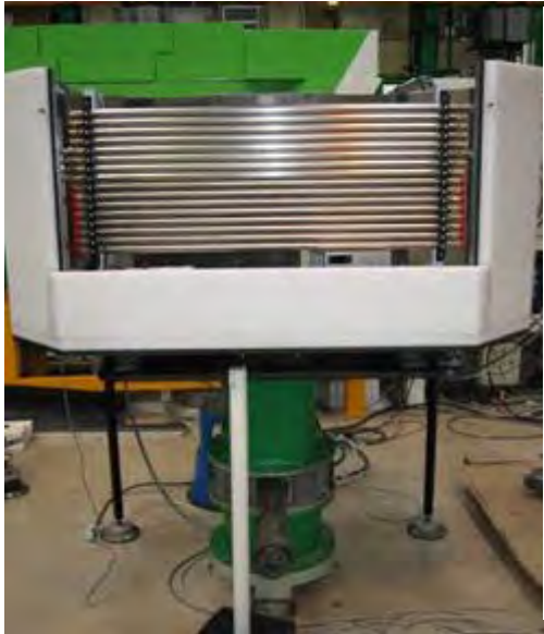
Figure 2 left: new 2D multidetector of G6.1 (LLB); right: scheme of the stress induced magnetic texture measured on G6.1
