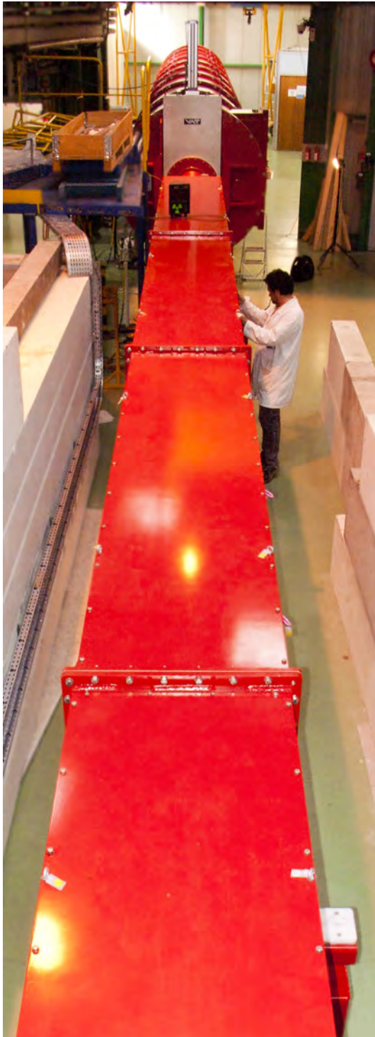
View of PA20 from the top of the casemate. The 16m long collimator is in the foreground and the detector tank in the background.
