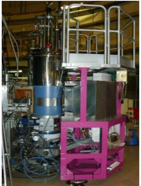
Figure 3: Polarized neutron diffractometer 5C1-VIP equipped with a PSD detector (Position Sensitive Detector)
