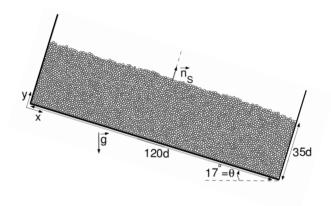
FIG. 1: A typical simulated granular pile of 4000 disks whose diameters are polydispersed at 20%, inclined at an angle  $\theta = 17^{\circ}$  in the gravity field  $\vec{g}$  with the xy-frame linked to the bottom of the box and the unity vector normal to the free surface  $\vec{n}_S$ .
