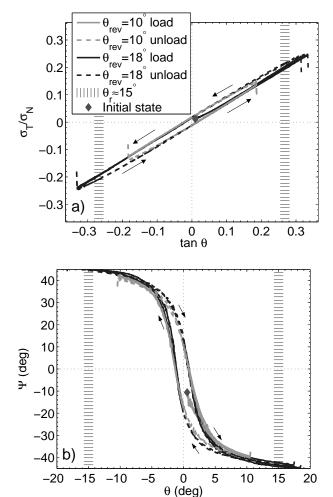
FIG. 7: Shear stress ratio  $\sigma_T/\sigma_N$  (a) and principal stress direction  $\Psi$  (b) as a function of the pile slope  $\theta$  during cyclic rotations for small ( $\theta_{rev}=10^\circ$ ) and large ( $\theta_{rev}=18^\circ$ ) amplitudes. The vertical lines correspond to the value of  $-\theta_r$  and  $\theta_r$ . The initial state is represented by a diamond.
