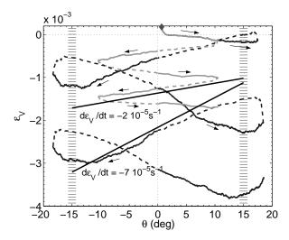
FIG. 8: Volumetric strain  $\epsilon_V$  as a function of the pile slope during small and large cycles (same symbols as figure 7). The two lines are indications of the compaction rate  $d\epsilon_V/dt$  for  $\theta_{rev}=10^\circ$  and  $\theta_{rev}=18^\circ$ .
