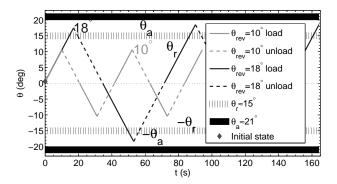
FIG. 2: Temporal plot of the surface slope  $\theta(t)$  of the granular pile during the loading-unloading solicitations for  $\theta_{rev} = 10^{\circ}$  (in gray) and  $\theta_{rev} = 18^{\circ}$  (in black). The horizontal lines, with a thickness equal to the size of the fluctuations among 50 realizations, correspond to the repose and avalanche angles  $\theta_r$  and  $\theta_a$ . The initial state of the pile just before the cycles start is represented by a diamond.
