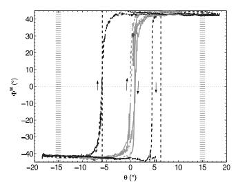
FIG. 14: Principal stress direction in the weak contact network  $\Psi^w$  as a function of the pile slope during the cycles for small and large amplitudes (same symbols as figure 7).
