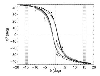
FIG. 13: Fabric anisotropic direction of the strong contact network  $\Phi^s$  as a function of the pile slope during successive loading-unloading cycles for small and large amplitudes (same symbols as figure 7).
