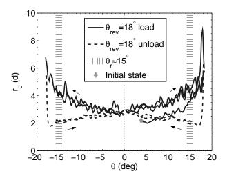
FIG. 6: Size of the correlated clusters of critical contacts  $r_c$ , slide-averaged over 1°-intervals as a function of the slope angle  $\theta$  during the successive cyclic solicitations for  $\theta_{rev} = 18^{\circ}$ .
