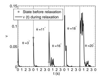
FIG. 4: Relaxation of the density of critical contacts  $\nu$  as a function of time in 5 granular piles inclined at different angles  $(\theta=3^{\circ},11^{\circ},16^{\circ},18^{\circ},20^{\circ})$  after the rotation was stopped at t=0. The state of the pile just before the relaxation starts is represented by a circle.
