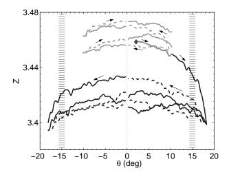
FIG. 10: Coordinancy of the grains Z slide-averaged over 1°-intervals as a function of the slope of the pile for successive small and large cycles (same symbols as figure 7).
