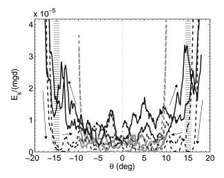
FIG. 9: Kinetic energy  $E_k$  averaged over all the grains and slide-averaged over 1°-intervals, normalised by the typical potential energy of a grain of mass m for a height d, as a function of  $\theta$  for  $\theta_{rev} = 10^{\circ}$  and  $\theta_{rev} = 18^{\circ}$  (same symbols as figure 7).
