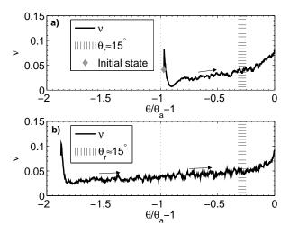
FIG. 3: Density of critical contacts  $\nu$  averaged over 50 simulations (a) during the first loading starting from  $\theta \simeq 0^{\circ}$  and (b) during one large cycle, starting from a pile inclined at  $-\theta_{rev} = -18^{\circ}$ , when varying the slope inclination towards the avalanche angle.
