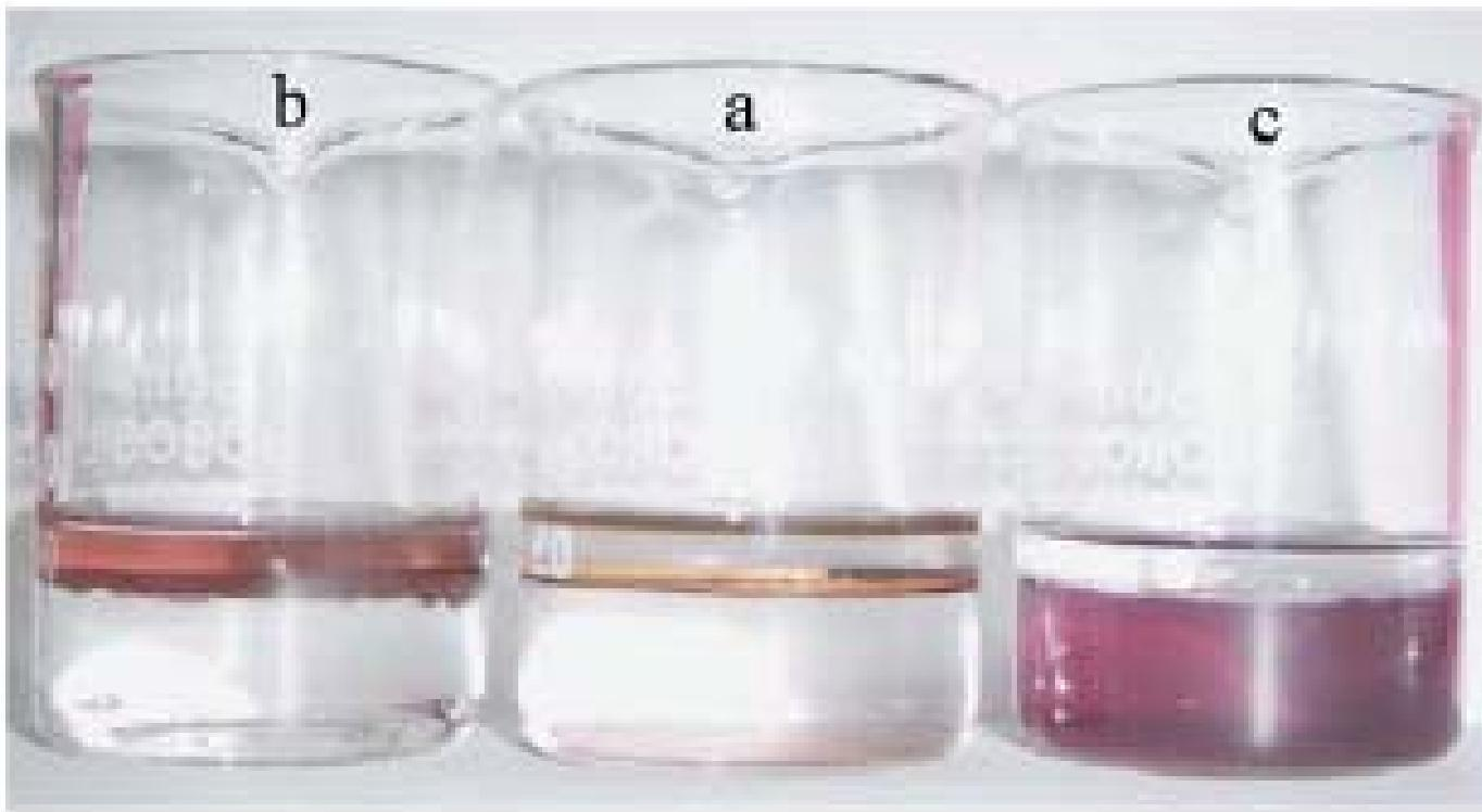
Nanocrystalline film of Au formed at the toluene–water interface.
