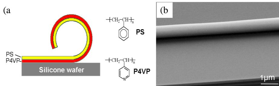
**Fig.1** (a) Structure of a polymer bilayer which undergoes self-rolling in a water solution of an alcohol or an acid. (b) Scanning electron microscopy of a micron-wide tube.
