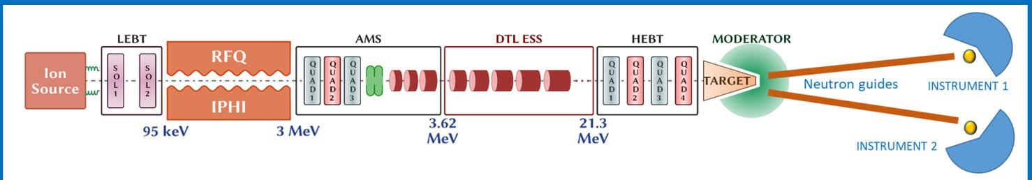
A high intensity ( $I_{\text{peak}} = 100\text{mA}$ ) pulsed proton beam is sent on a beryllium target. Via stripping reactions, fast neutrons are produced. Neutrons are thermalized at temperatures of 20 to 300K to have wavelengths from 1 to 20 Å adapted to studies in chemistry and physics of condensed matter.
