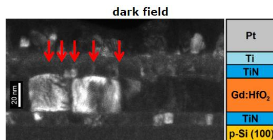
Figure 2: ~ 30 nm granularity in HfO 2 MIM structure on silicon 5
