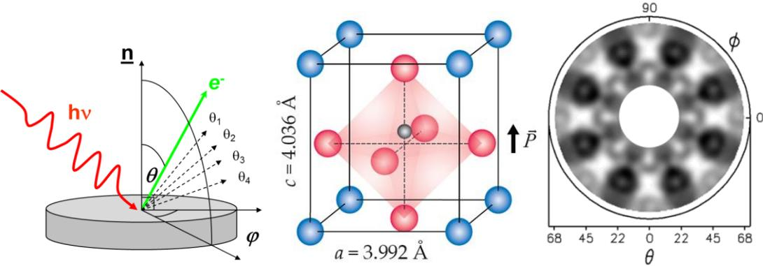
(a) Schematic XPD experiment (b) Tetragonal  $BaTiO_3$  with Ti (grey) off-centering (c) Ti 2p XPD data from single crystal  $BaTiO_3(001)$  allowing measurement of the Ti displacement in the surface unit cell.
