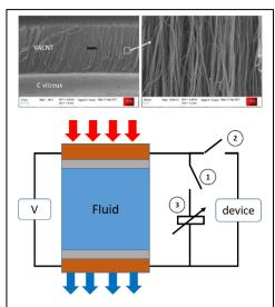
Figure 1 (Top) SEM images of vertically aligned carbon nanotubes grown on glassy carbon surface (courtesy of LEDNA/NIMBE/IRAMIS/CEA). (Bottom) A schematic illustration of a thermally chargeable ionic supercapacitor. ① Switch connecting a (charging) resistance ③ to the TISC cell. ② Switch connecting the electronic device to the TISC.
