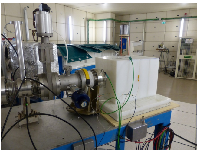
Polyethylene moderator (white cube) containing a Be target on which protons of energy 3MeV are sent. The Time of flight detector is set in the back, 8m away from the moderator.
